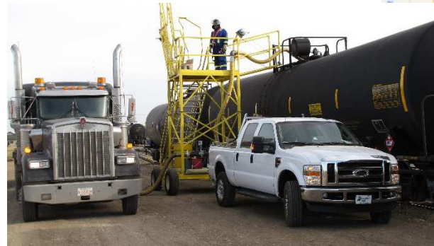
Towable gantry and 8 railcar siding capacity
